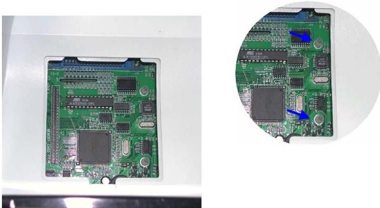
4. Check the pins where the memory is to be connected to, then plug the memory card onto the mainboard.
