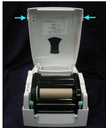
2. Take off the media roll spindle. Open and remove the plastic cover on the inner base.
