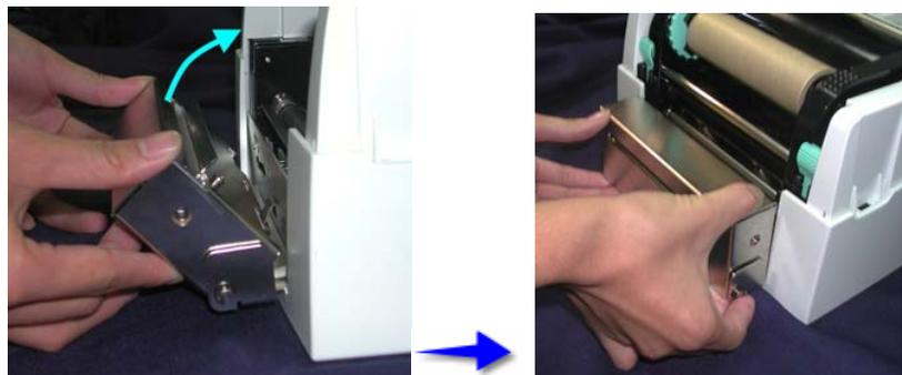
9. Close the mechanism to complete the cutter module installation.
