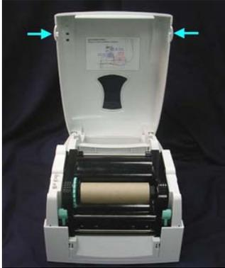
A top-down view of the printer with its top cover open. Two red arrows point to the hinges of the top cover.                                                                                                                                                                                                                |
