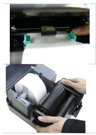
5. Adjust the label guide to fit the width of the media.
