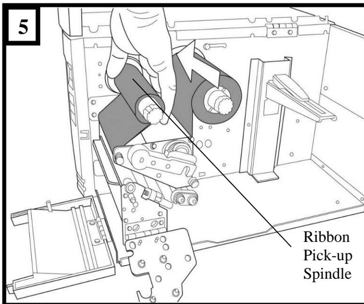
7. Turn the pick-up spindle to ensure the ribbon is tightly wound.
