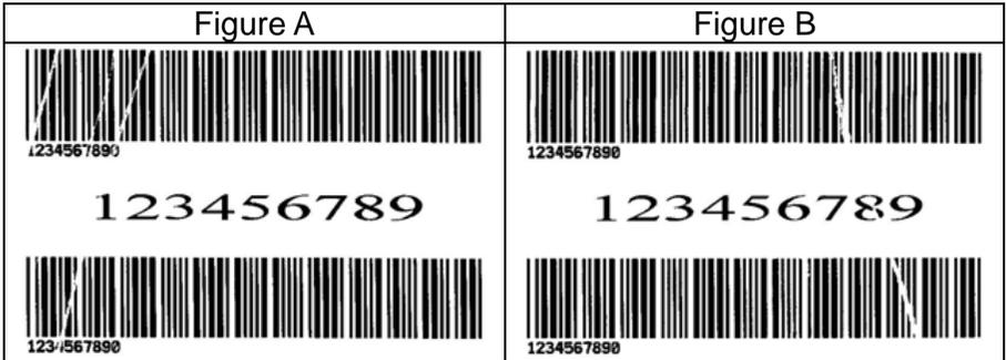
Once the printouts as above appear, the possible cause may be the unequal positions of Ribbon Bracket, which needs to be adjusted properly to make its heights equally the same at both sides. Steps to adjust are as below:
