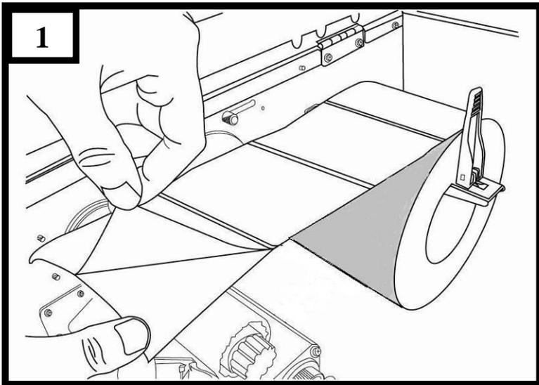
2. Lead the media backing paper through the print head module. (Figure 2)
