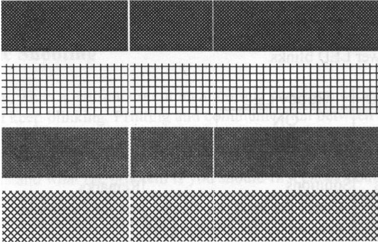
For unstable ribbon roll rotation, check the label path and make sure the head latch is securely closed.
