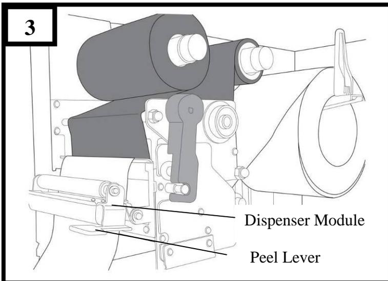
4. Close the peeler module using the peel-off mechanism release lever. (Figure 4)
