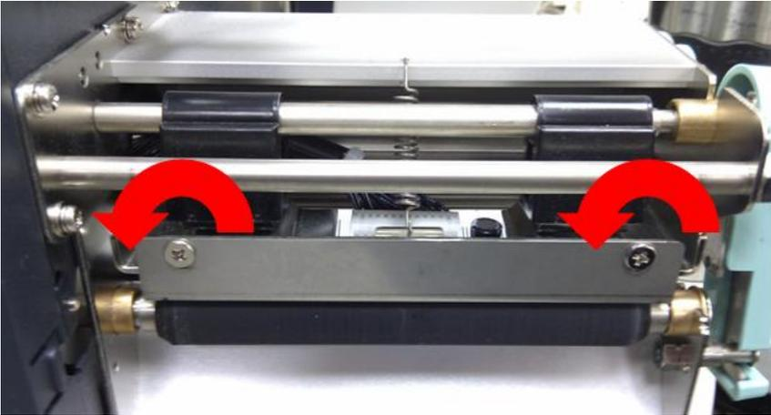
2. Make sure the Ribbon Bracket is at its lowest position first; then tight up the screws by rotating clockwise.
