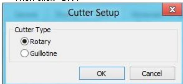
Check on the radio button, “Guillotine” if there’s Guillotine Cutter installed. Then click “OK“:
