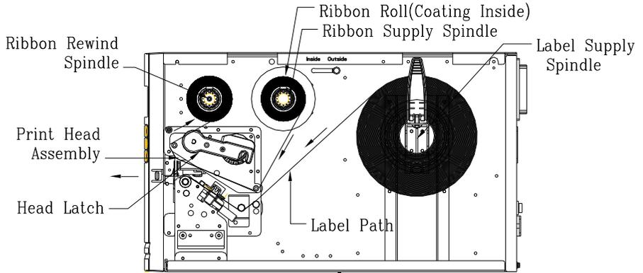
3. If ribbon wound ink-side in is in use, pull and move the SHAFT RIBBON ADJ to "Inside". Then install the ribbon:
