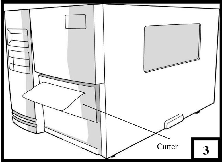
**Note:** The FEED button does not make the printer cut. To enable Cutter function, set by the LCD panel
