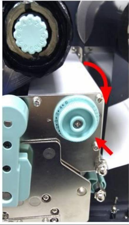
Once the desired quality has been reached, please make note on the new setting of the Fine Adjustment Knob and the type number of ribbon been used in this printing task for future reference.
