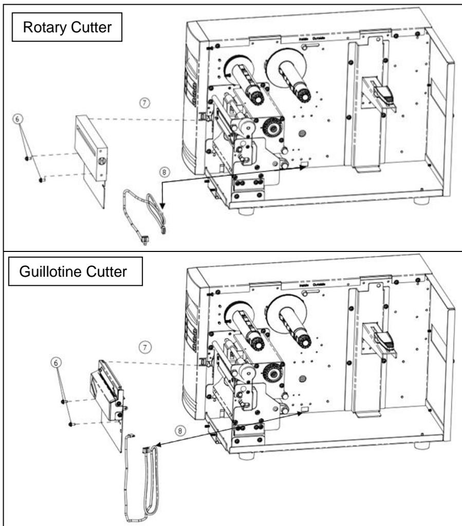
6. Thread the cutter cable (8) through hole and route it to the **JP16** connector (CUTTER) on the **X-1000VL/ X-2000V/ X-2000V Zip** main boards, or to the **JP14** connector (CUTTER) on the main board of **X-2300/ X-2300Z/ X-2300E/ X-2300ZE/ X-3200/ X-3200Z/ X-3200E/ X-3200ZE**.
